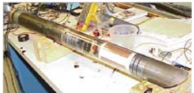
Prototype of HDD drill head with obstacle-detection capability being tested at GTI facilities.
